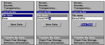
These figures (left to right) show the menu sequence for naming and saving a GPS Data File from the unit's memory to an MMC.
